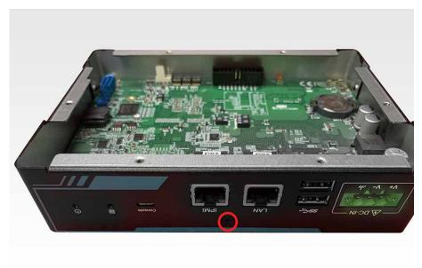
**Step 2** Remove two pcs F-M3x4L screws for rear panel.
