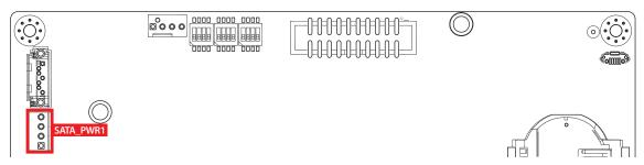
The VAC-1000 is also equipped with one SATA power connectors. It supports 5V (Up to 2A) and 12V (Up to 2A) currents to the hard drive or SSD. The pin assignments of SATA PWR1 is listed in the following table:
