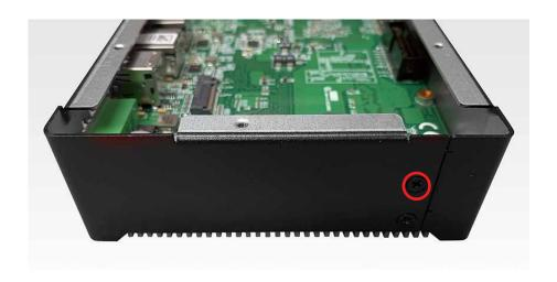
**Step 4** Remove four pcs PH-M3x4L screws on the motherboard.
