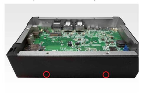
**Step 3** Remove four pcs F-M3x4L screws for both sides.
