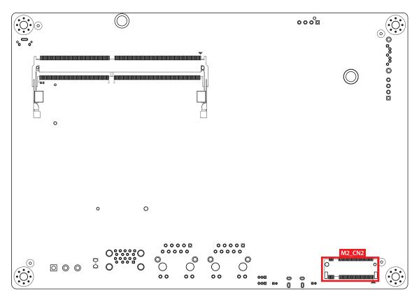
The supported M.2 module card type is 2280. M2\_CN2 is pre-installed with the Hailo- $8^{\,\text{TM}}$ /Lightspeeur® Al Accelerator Card. The pin assignments of M2\_CN2 in the following table :
