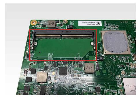
**Step 6** Make sure the RAM module is locked by the memory slot.
