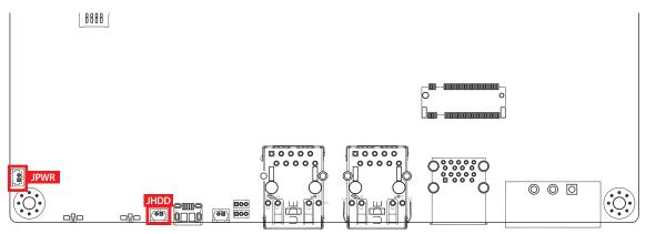
These pin headers can be used as a backup for the following functions : Power LED indicator, Hard Drive LED indicator.
