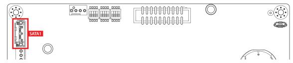
There is onboard high performance Serial ATA III (SATA III) on VAC-1000. It supports higher storage capacity with less cabling effort and smaller required space. The pin assignments of SATA1 is listed in the following table:
