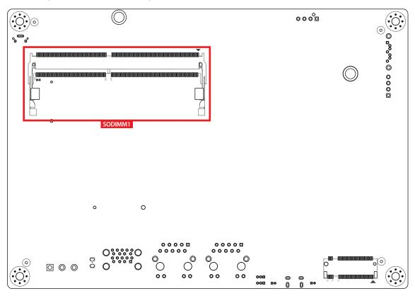
The SO-DIMM connector is suitable for a DDR4 memory module. Please refer to Appendix C for certified memory modules.
