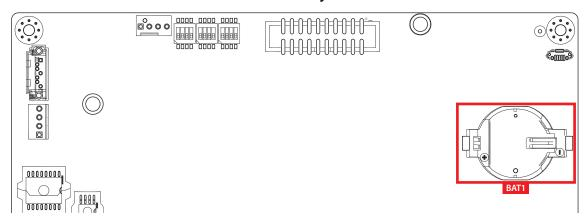
System has a built-in CR2032 battery holder that allows the real-time clock to keep the clock running remain operational when the system is disconnected from power.
