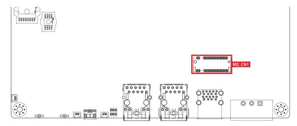
The supported M.2 module card type is 2280. The pin assignments of M2\_CN1 in the following table :
