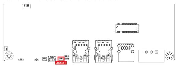
This is used to execute hardware system reset function.
